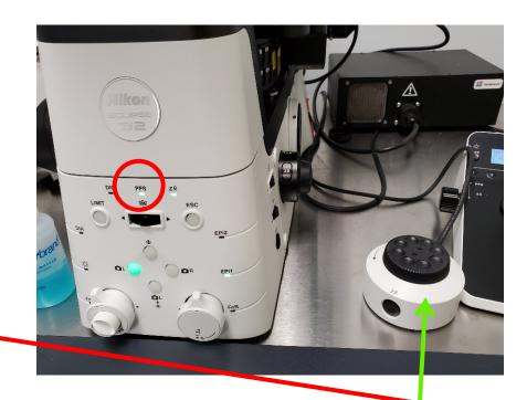
Blinking PFS LED: Not locked, use the z focus knob
