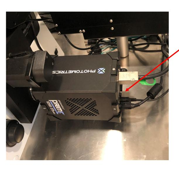
The initializing light will blink while the camera is initializing. When it stops blinking the computer can be turned on.
