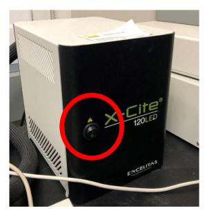
Press the large black knob to turn the LED on and off. Turn the knob to change the LED intensity 1 – 100%
