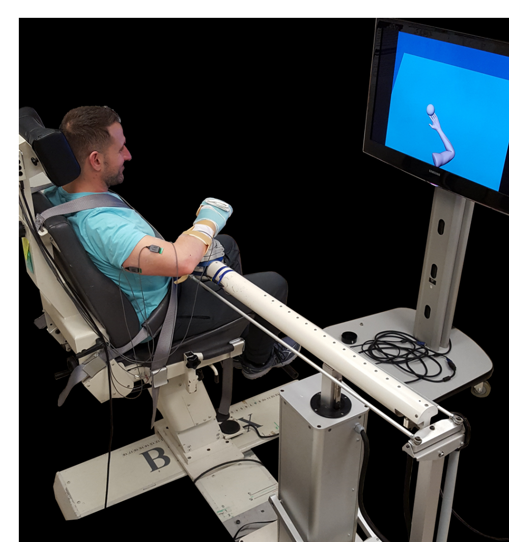
Figure 2: Experimental setup for dynamic measurement of reaching function and flexion synergy.
