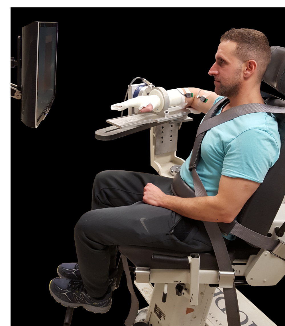
Figure 1: Experimental setup for isometric measurement of shoulder and elbow strength
